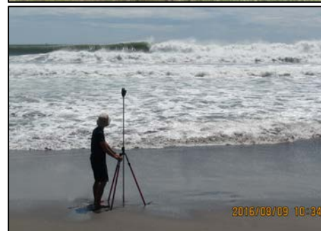
Wave measurements using pressure sensor and total station
