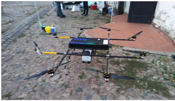
An eight-copter drone used for chemical decontamination.
