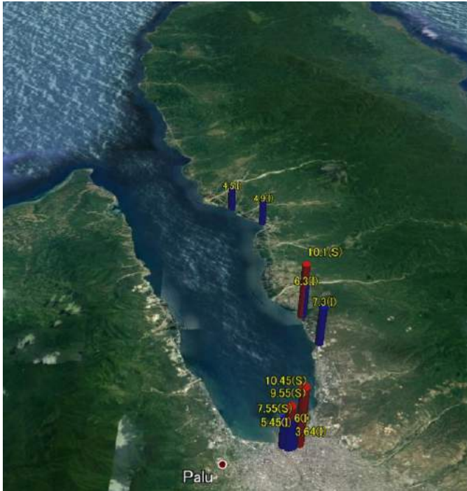
Figure1. The result of field survey data showing the tsunami heights of splash wave (red color) and flow depth (blue color) measured in Palu bay overlaid in Google earth, without tidal correction (Muhari et al, 2018 JDR submitted).
