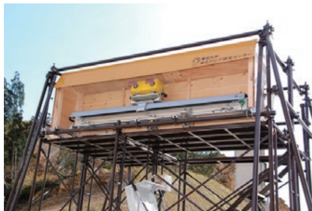
Fig. 2.11 GB-SAR system installed at the Arato-zawa site
