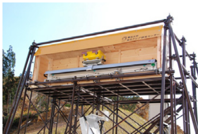
Fig. 2.11 GB-SAR system installed at the Arato-zawa site
