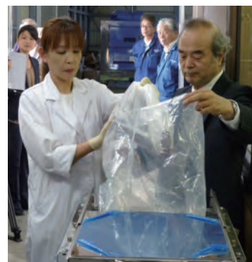
In the past, measuring the concentration of a radioactive substance on products required the preparation of samples by chopping up the products into pieces. However, the Research Center for Remediation Engineering of Living Environment Contaminated with Radioisotopes has developed new machine that doesn't require a such a sample to detect radiation; this shortens the time required for preparation. Professor Ishii, on the right, is in charge of the "06 project to develop countermeasures against radioactive substance contamination" at Tohoku University's organization for Disaster Recovery.
