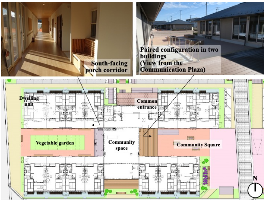
Figure 21-1. Living-access Housing (O Housing, Kamaishi City, Iwate Prefecture) Design: Chiba University Architectural Planning Office + Daiwa House Industry Co., Ltd. Design support: Tohoku University Onoda/Tsukada Laboratory
